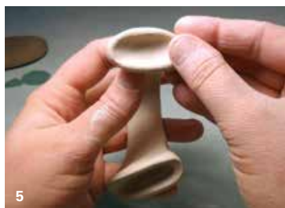
5 Make the thicker ends of your handles concave by pressing in with your thumb.
