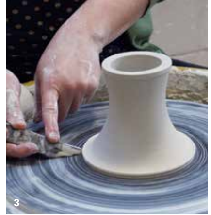
3 Throw a stem that is bottomless and tapered in at the middle.
