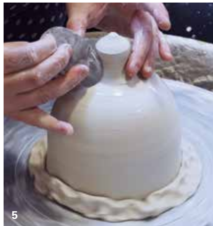
5 Throw a knob on top of the lid using a small piece of clay.
