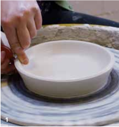
1 Throw a plate that is \frac{3}{8} inch thick, 5 inches wide, and 1\frac{1}{2} inches tall.
